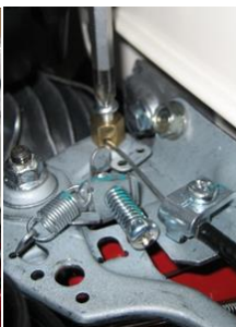
3 ATTACH THE THROTTLE SIRGA
