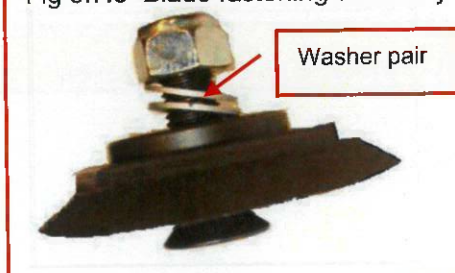
Fig 6.7.3 Blade fastening assembly
